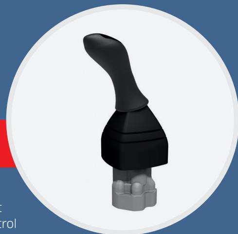
Our PV series valves are pressure-reducing type pilot valves that allow operators to simultaneously control spools of multiple control valves as well as the tilting angle of variable displacement pumps. The operational torque can be reduced to meet your requirements (Patent registered), while the small operational force enables minute control, reduced pressure drop and quick response.
