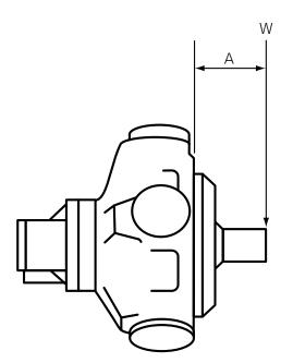
**A** = Distance from mounting face to load centre (mm)
